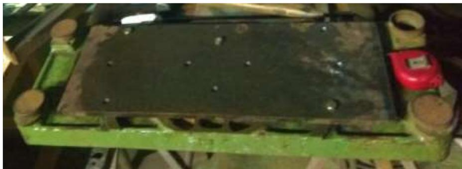
**Figura 8.** Chapa aparafusada na mesa
